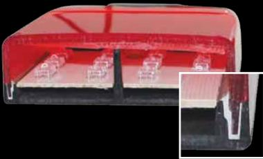
The lamp is then susceptible to chemical attack, enlarging the crack(s) and may lead to failure of the seal. HELLA's gluing process does not place any undue stress on the plastic material, therefore will remain sealed for many years.
